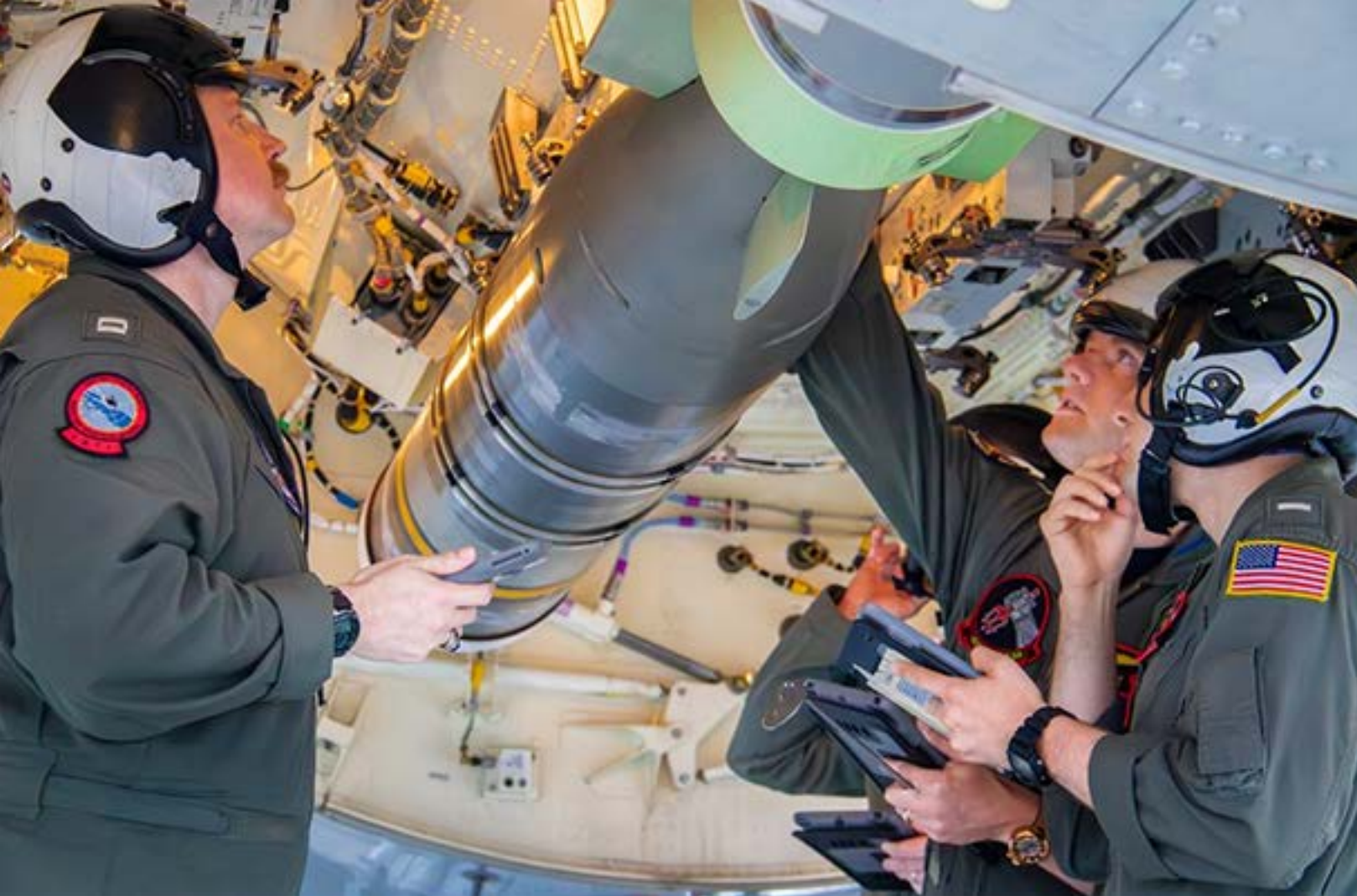
(TOP) NAVAL AIR STATION WHIDBEY ISLAND, Wash. (Aug. 1, 2023) -- Naval Aviators and Naval Flight Officers attached to Patrol Squadron (VP) 46, the 'Grey Knights,' conduct checklist items to ensure the MK 54 Warshot Torpedo is secured and supported inside the weapons bay of a P-8A Poseidon at Naval Air Station, Whidbey Island, Washington, Aug. 1 2023. VP-46 was tasked with conducting a surface weapon test of the MK 54 Warshot Torpedo to evaluate the performance and effectiveness of the weapon's inventory. (U.S. Navy photo by Mass Communication Specialist 2nd Class Jacquelin Frost.)
