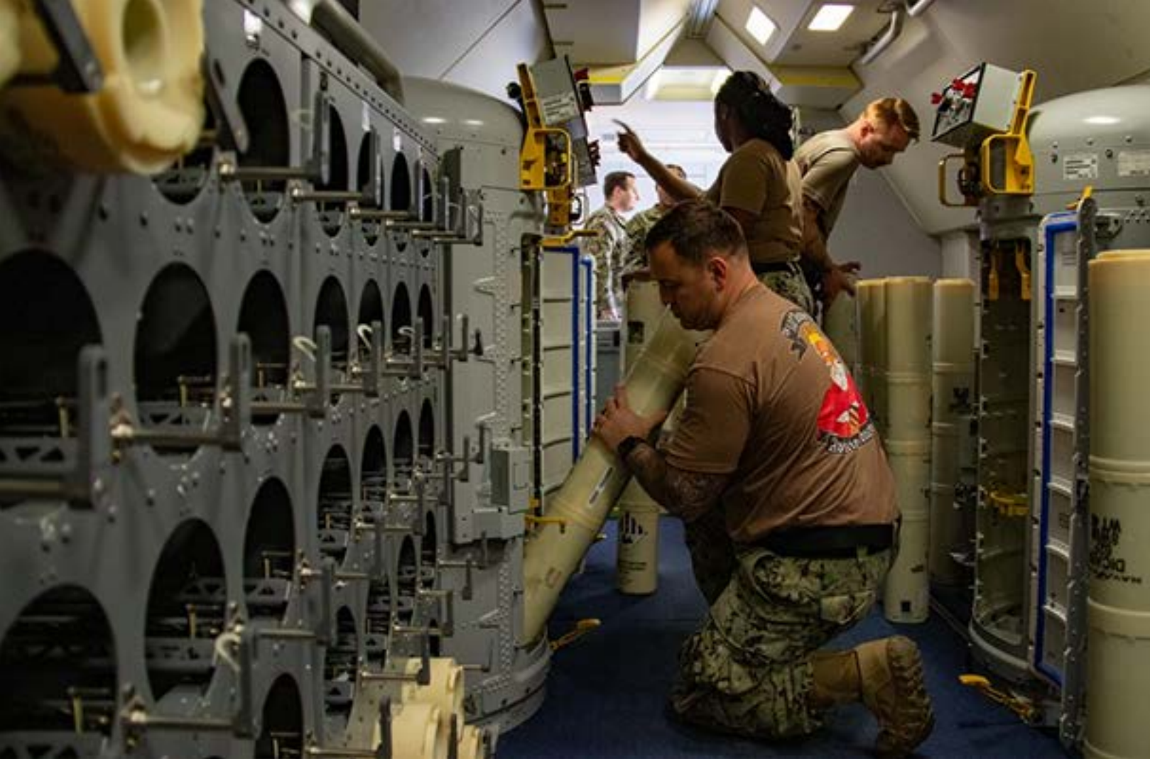
(TOP) ROYAL AIR FORCE LOSSIEMOUTH, United Kingdom (July 13, 2023) – Sailors assigned to the ‘Golden Swordsmen’ of Patrol Squadron (VP) 47, load sonar buoys onto a P-8A Poseidon at Royal Air Force (RAF) Lossiemouth, July 13, 2023. VP-47 is currently deployed to the U.S. 6th Fleet in support of naval operations to maintain maritime stability and security in order to ensure access, deter aggression and defend U.S., allied and partner interests. (U.S. Navy photo by Mass Communication Specialist 1st Class William Sykes/Released)
