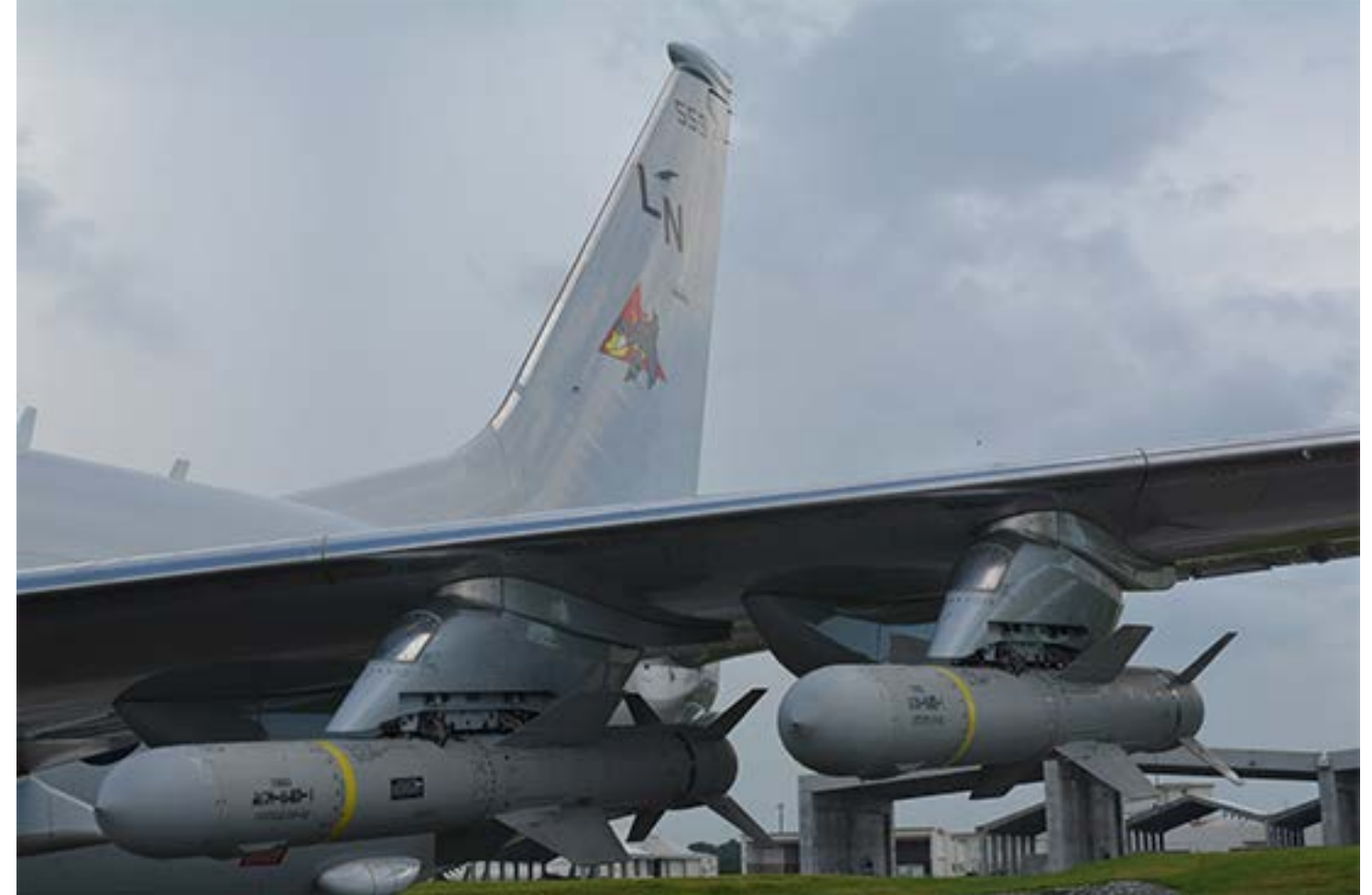
We couldn't have asked for a better sight . The A/U/RGM-84 Harpoon is an all-weather, over-the-horizon, anti-ship missile system that provides the Navy with a common missile for air and ship launches. Courtesy VP-45.
