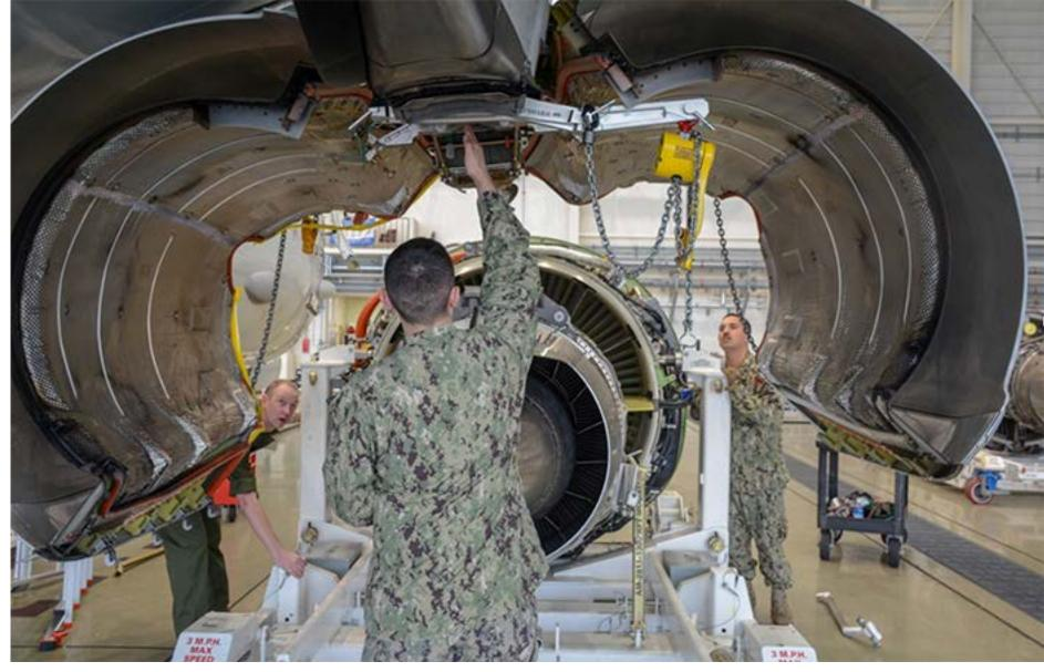
Photo by MCSN Thomas A. Higgins. Maintainers of VP-45, replace an engine on a P-8A.
