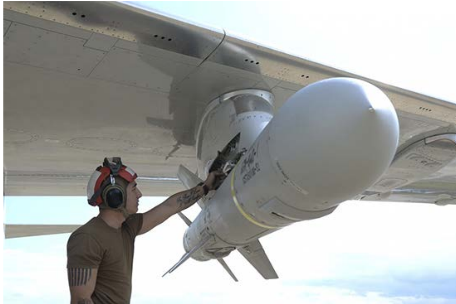
SIGONELLA, Sicily (Oct 08, 2019) Aviation Ordnanceman 3rd Class Phillip Marotta, assigned to the "Skinny Dragons" of Patrol Squadron (VP) 4, installs an AGM 84D Harpoon missile during a monthly task force weapons proficiency check. VP-4, forward deployed to the U.S. 6th Fleet area of operations is assigned to Commander, Task Group 67, responsible for tactical control of deployed maritime patrol and reconnaissance squadrons throughout Europe and Africa. (U.S. Navy photo by Mass Communication Specialist 2nd Class Juan Sua/Released)
