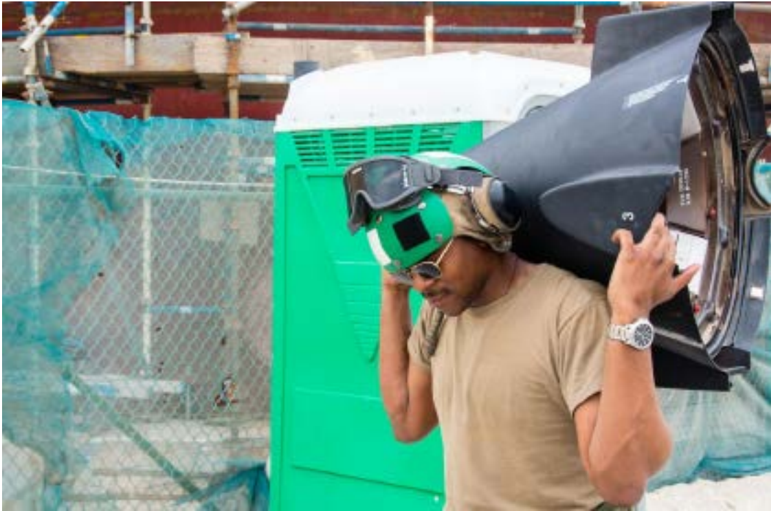
Some of the most difficult maintenance revolves around the four propellers of the Allison T-56 turbo-prop engines on the P-3C. This motivated sailor is carrying one of the propeller nosecones, known as a “spinner.” Photo courtesy of VP-1.
