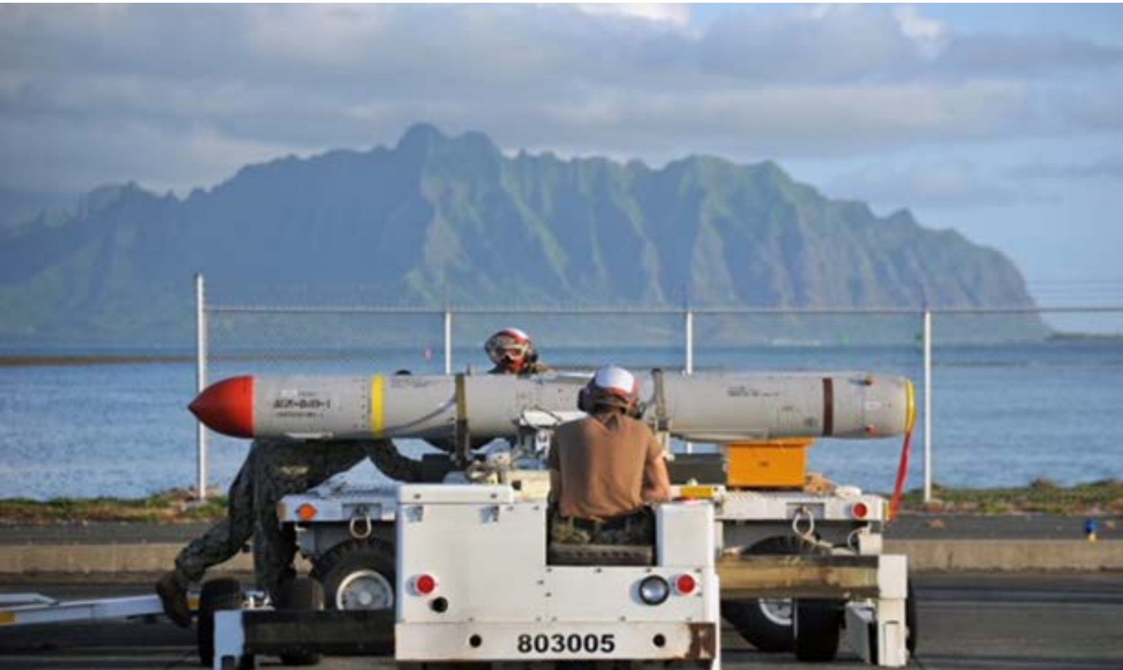
KANEOHE BAY, Hawaii (July 12, 2018) — Sailors assigned to the “Golden Swordsmen” of Patrol Squadron 47 use a MHU-83 Munitions Handling Unit to load a AGM-84D Harpoon missile onto a P-8A Poseidon aircraft on Marine Corps Base Hawaii during Rim of the Pacific (RIMPAC) exercise. (U.S. Navy photo by Mass Communication Specialist 1st Class Kevin A. Flinn/Released)
