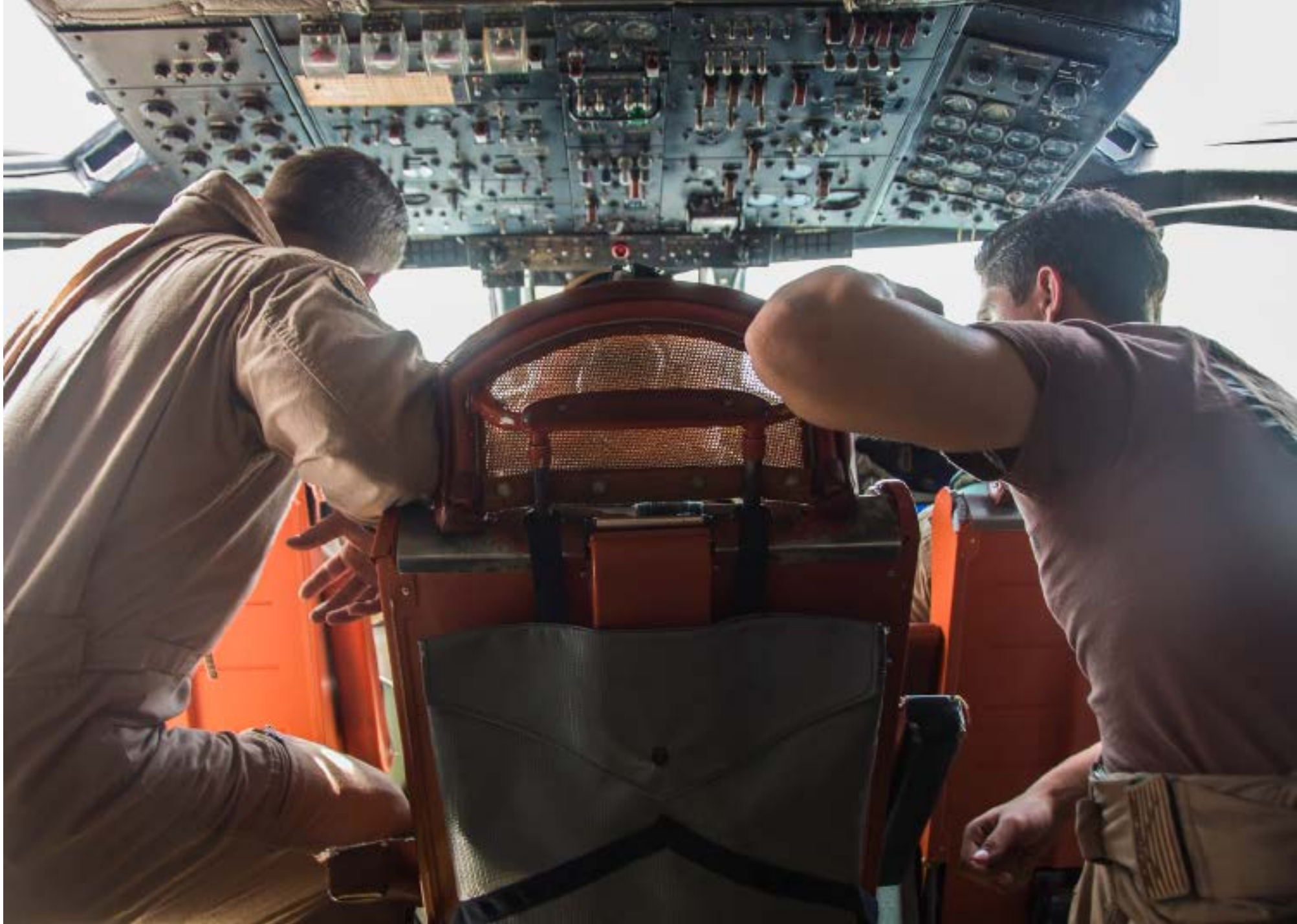
The P-3C Orion’s cockpit is unique in that it is large and can easily fit 5-6 people while cruising along at altitude. Overhead windows in conjunction with large side windows improve the VFR scan capability of a P-3C’s flight crew. Having additional personnel in the front of the plane also improves the situational awareness of the crew, especially on long 10 hour plus missions, often throughout the night. Seen here is the cockpit known as the “flight station” in the P-3C. Two pilots and a Flight Engineer (AWF) make up the flight station composition. Photo courtesy of VP-1.
