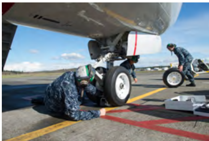
OAK HARBOR Wash. (May 5, 2017). Patrol Squadron FOUR (VP-4) maintenance personnel perform checks on the nose wheel of the P-8 Poseidon. VP-4 was declared safe to operate the new maritime patrol and reconnaissance aircraft after a weeklong series of inspections and evaluations. (U.S. Navy photo by Mass Communication Specialist 3rd Class Juan Sua).
