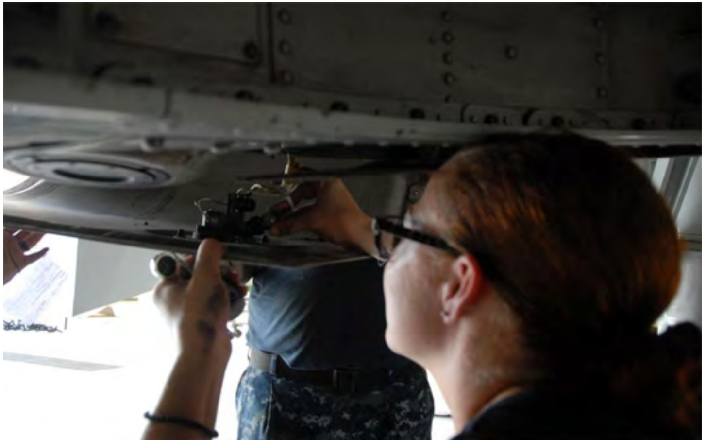
AE2 Shannon Strange connects a ground illumination light Sept. 8 onto the underside of a P-8A Poseidon aircraft in VP-16's hangar bay. The P-8A must undergo frequent maintenance in order to perform at the highest level possible.
