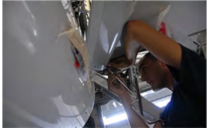
AM3 Corey Parker checks a P-8A for signs of corrosion. Every inch of a naval aircraft such as the P-8A Poseidon must be visually checked for corrosion to maintain airframe integrity.
