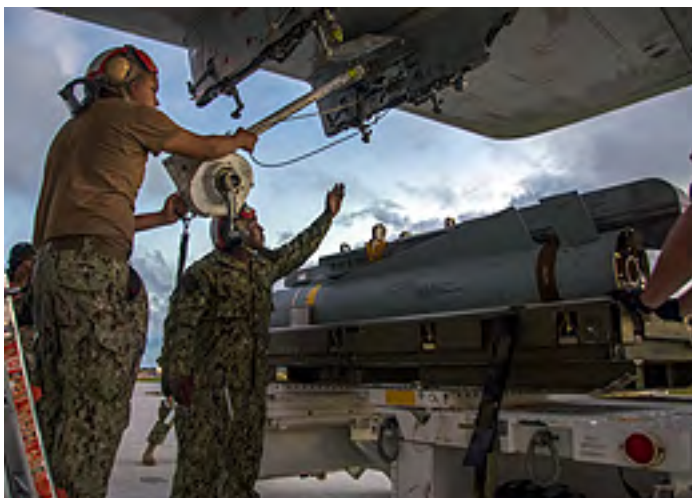
GUAM (September 13, 2016) - Aviation Ordnanceman 3rd Class Donta Stone and Aviation Ordnanceman Airman Ederson Corpus assigned to Patrol Squadron (VP) 46 load an AGM-65F Maverick air-to-surface missile on a P-3C Orion aircraft during Exercise Valiant Shield. Valiant Shield focuses on integrated joint training among U.S. military forces, enabling real-world proficiency in sustaining joint forces and in detecting, locating, tracking and engaging units at sea, in the air, on land and cyberspace in response to a range of mission areas. (U.S. Navy photo by Mass Communication Specialist 3rd Class Alexander Cole/Released)
