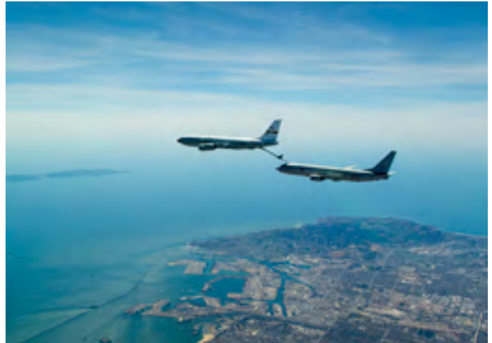
EDWARDS AIR FORCE BASE, Calif. -- A U.S. Navy P-8 Poseidon conducts aerial refueling tests with a U.S. Air Force KC-135 Stratotanker over different parts of Southern California, to include the Sierra Nevada mountains, Western Mojave Desert, greater Los Angeles, and the Pacific Ocean. (U.S. Air Force photo by Christopher Okula)
