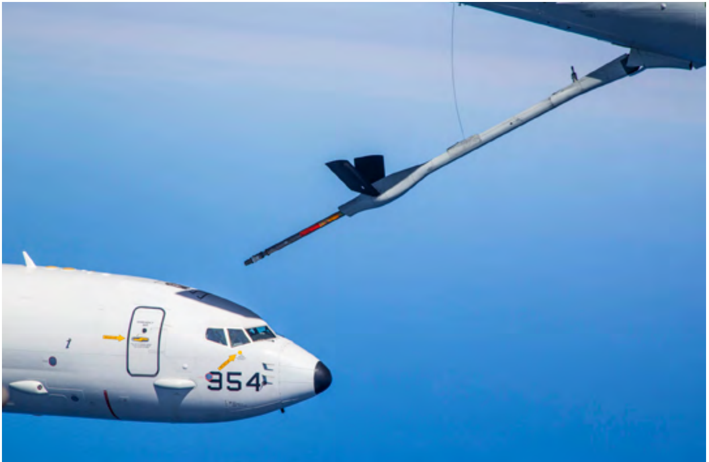
EDWARDS AIR FORCE BASE, Calif. -- A U.S. Navy P-8 Poseidon conducts aerial refueling tests with a U.S. Air Force KC-135 Stratotanker over different parts of Southern California, to include the Sierra Nevada mountains, Western Mojave Desert, greater Los Angeles, and the Pacific Ocean. (U.S. Air Force photo by Christopher Okula)
