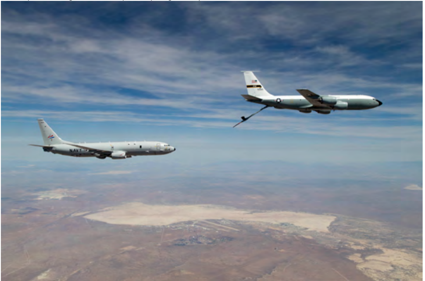
EDWARDS AIR FORCE BASE, Calif. -- A U.S. Navy P-8 Poseidon conducts aerial refueling tests with a U.S. Air Force KC-135 Stratotanker over different parts of Southern California, to include the Sierra Nevada mountains, Western Mojave Desert, greater Los Angeles, and the Pacific Ocean. (U.S. Air Force photo by Christopher Okula)
