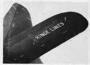
One unique feature of P2V-2 is the varicam tail, which really gives it two elevators and increases its flight maneuverability
