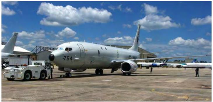
Photo courtesy of VP-30. VP-30 maintenance personnel use a tow vehicle to back a P-8A Poseidon aircraft into its parking spot at Cecil Airport.
