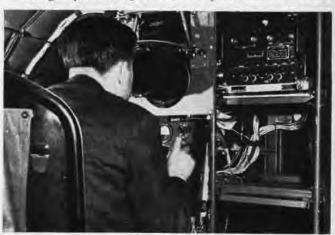
Neptunes carry plenty of radar and radio gear; this picture shows camera installed for photographing traces on scopes
