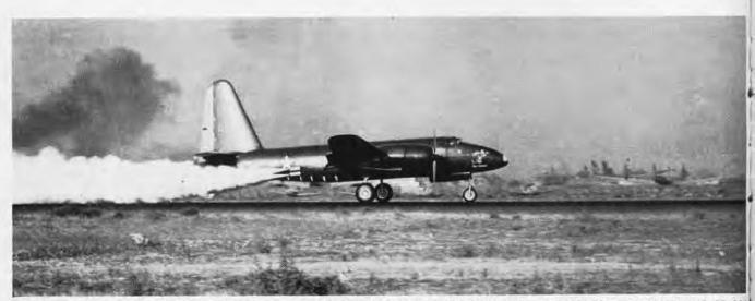
TRUCULENT TURTLE, NAVY'S MOST FAMOUS AIRCRAFT, TAKES OFF WITH SHORT RUN BY USING JATO. BELLY STRIPES MEASURE DUMPING OF GAS
