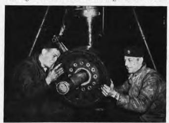
Two mechanics of VP-ML-7, J. L. Carpenter AD1, and L. G. Judas, ADC, change brake expander tube on wheel of a P2V-2
