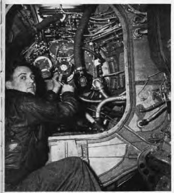
**VP-ML-8** man demonstrates accessibility of rear of Neptune's engine for repairs; this feature makes the plane popular
