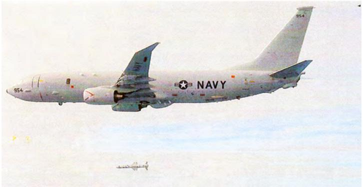
Armament of the P-8A Poseidon can include the AGM-84D Harpoon Block IC anti-ship missile seen here during recent trials. Limited to nations with sufficient budgets, at US \$130-180M each, the P-8A is well beyond the reach of most countries considering the new MPA acquisitions. Photo courtesy of Boeing.
