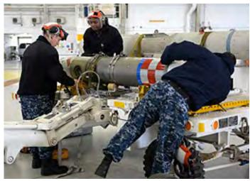
Photos by MC2 Clay Whaley. Aviation ordnancemen assigned to the "Fighting Tigers" of VP-8 prepare to transfer a Recoverable Exercise Torpedo from the weapons cart to the P-8A bomb bay during the recent Conventional Weapons Technical Proficiency Inspection.
