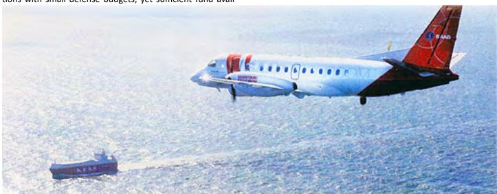
Based on the 340 regional airliner, the Maritime Security Aircraft (MSA) is a multi-role surveillance aircraft for detection, classification, and identification of maritime contacts. The X-band radar carried by the aircraft is Telephonics RDR-1700B radar which uses SAR and ISAR (Inverse SAR) modes to provide a maximum image resolution of 1m. Photo courtesy of Saab.
