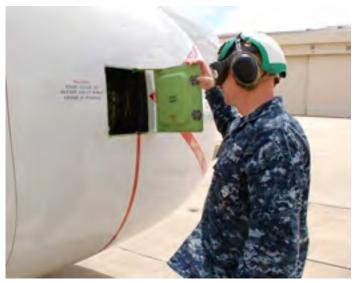
Photos by Clark Pierce. AD2 Mauricio Granato unlatches an engine panel on a P-8A Poseidon that is part of the aircraft's pre-flight inspection.
