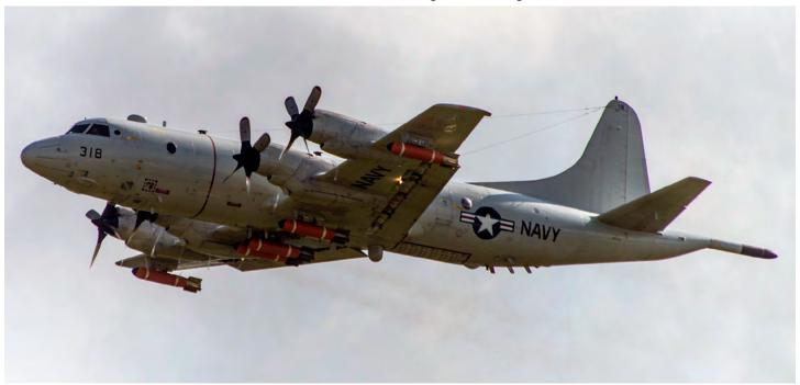
Photo courtesy of VP-30. This P-3 Orion assigned to VP-30, takes off from NAS Jacksonville with a full load of practice MK 65 Quickstrike mines attached to underwing pylons and the fuselage.
