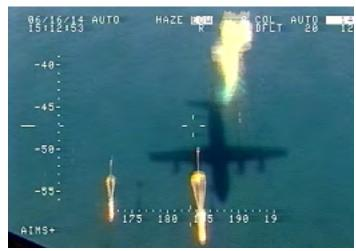
Photo courtesy of VP-30. A camera on board a P-3C Orion views launched MK 65 Quickstrike mines as they descend via parachute into the ocean.
