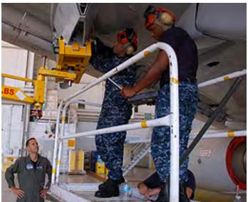
Photo by Clark Pierce. (From left) VP-45 Commanding Officer Cmdr. T.J. Grady observes AO2 Chase Dellinger and AO2 Gil Mine as they install a wing rack and pylon onto a P-8A in Hangar 511 at NAS Jacksonville. The Poseidon features four wing pylons and two center line pylons for armament such as the Harpoon anti-ship missile, torpedoes and mines.
