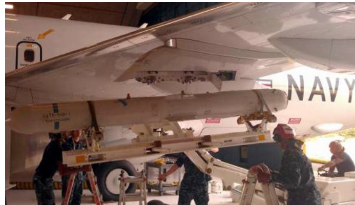
Photo by CWO5 Roddy Wiggins. VP-16 aviation ordnancemen prepare to load an AGM-84D Harpoon missile onto a P-8A Poseidon during training in Patuxent River, Md.
