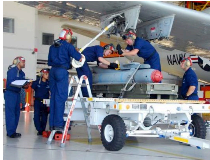
Photo by MC2 Clay Whaley. Aviation ordnancemen at VP-8 load an inert training weapon onto a P-3C Orion on Aug. 28 during the squadron's Conventional Weapons Technical Proficiency Inspection (CWTPI).
