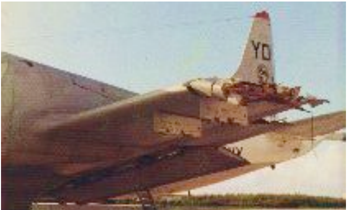
After landing in Midway Is after the collision. Notice the damage on the top of the tail.
