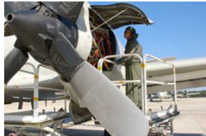
Photo by Clark Pierce. VP-26 Flight Engineer AWF1 Andrew Wray checks out the No. 2 Allison T-56 turboprop engine on the P-3C aircraft No. 926.
