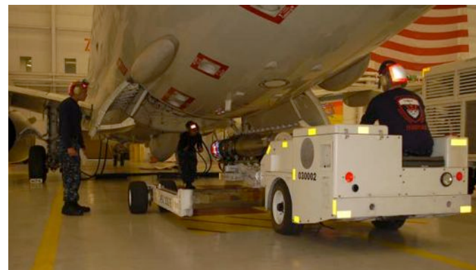
Photo by Clark Pierce. VP-16 ordnance riggers carefully direct the torpedo hoist driver as he slowly and precisely approaches the P-8A Poseidon internal bomb bay.
