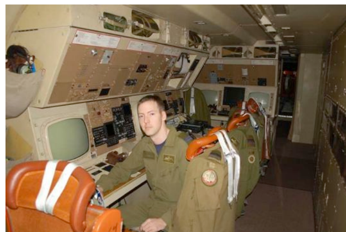
Photo by Clark Pierce. RCAF Lead navigator Capt. Chris Wattie explained that unlike the P-3C, the CP-140 navigator and sensor stations share side-by-side space within the fuselage.
