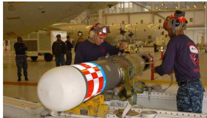
Photo by Clark Pierce. VP-16 ordnance shop riggers disconnect a MK 54 training torpedo from its transport cart and load it onto the weapons hoist.
