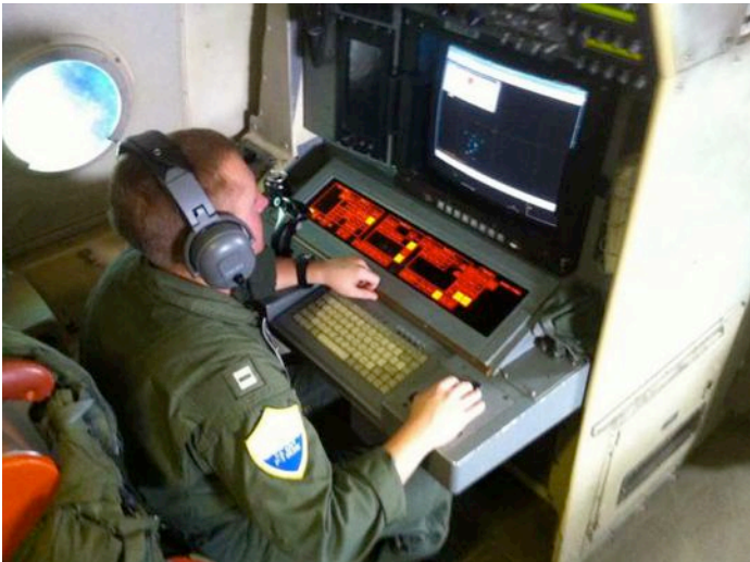
Photo by Lt. Ray Ratliff-VP-5 Mission Commander Lt. Timothy Clemens uses the P-3C's Automatic Identification System to analyze surface contacts and verify their compliance with international law.
