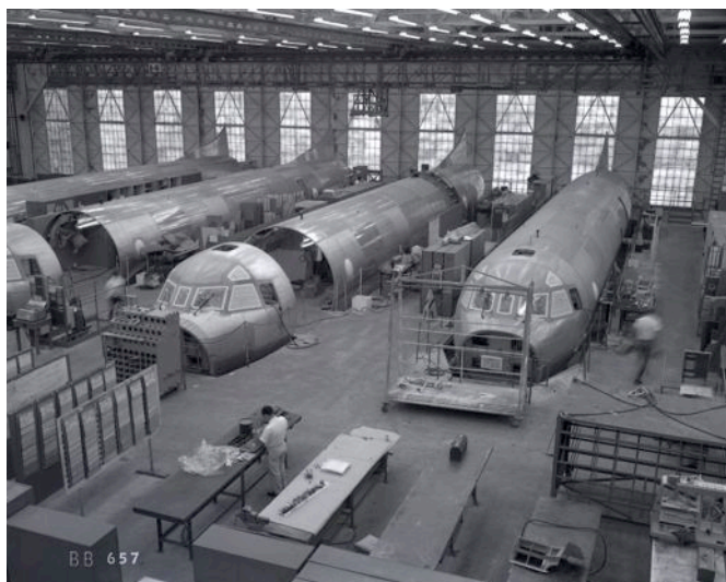
Lockheed Martin Aeronautics Company - Palmdale, CA. P-3 Orion Fuselage Final Assembly Burbank, CA Bldg. 306. Photo courtesy of the Lockheed Martin Corporation.
